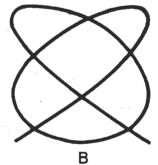
2 If the vertical frequency used to produce these Lissajous patterns is 1000 Hz, which has a horizontal frequency of 1200 Hz and which is 1250 Hz?
